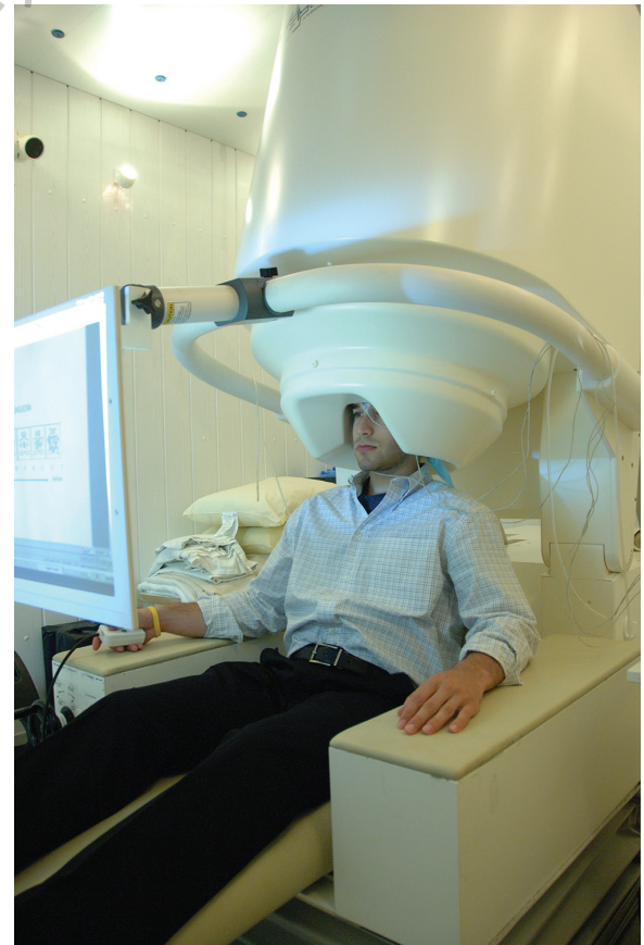
Magnetoencephalography measures brain activity by measuring small magnetic fields produced in the brain.
