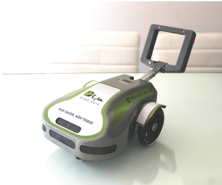
Lysa, a robotic guide dog for the visually impaired, created by Neide Sellin of VixSystem
